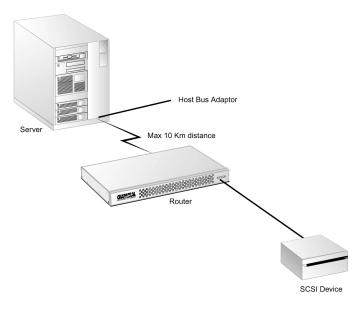
Figure 2-5. Simple loop configuration example
